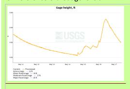
SUGAR CREEK AT CRAWFORDSVILLE, IN - USGS Water Data for the Nation The removal of a low-head dam on Sept. 7, 2021 caused water levels in Sugar Creek to drop abruptly and has periodically resulted in negative gage heights due to the reference datum for this monitoring station being approximately equal in height to the crest of the low-head dam prior to its removal.waterdata.usgs.gov
